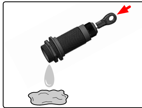
Drain the oil from the shock absorber.
